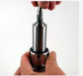
Insert cutter, while holding the cutter handle tighten the locking collar clockwise until the collet holds the tool.
