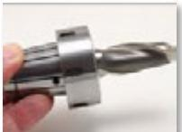
Fully insert cutter into the collet
