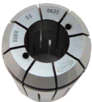
Coolant thru standard collet slots create a loss in pressure and flow control, allowing coolant to fly everywhere. The **Jet-Blast** option for SSER forces the coolant into the **Jet-Blast Ports** maintaining pressure and directing the coolant down the flutes of the cutting tool.
