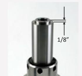
Turn collet until it stops or reaches 1/8" from the face of the chuck. Assemble loose,
