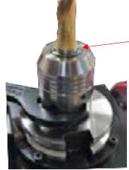
Body protruding approx. 1mm (0.040") from the lock nut at full torque.
