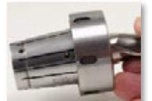
Once the pin is fully inserted pull out on the cutting tool so the back of the flat is tight against the pin
