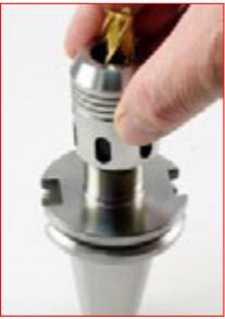
Grease Taper & Assemble the Lock Nut, Hand Tight
