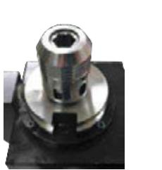
Remove the lock nut from the BC holder assembly, wipe off any dirt or existing grease from taper and inside the lock nut.
