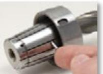
Insert Pin into the Pin Hole
