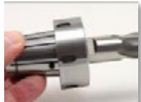
Insert cutting tool into the collet, cutter flat orientation to the pin hole as shown
