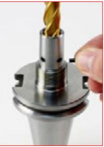
Insert the Hardened Dowel Pin
