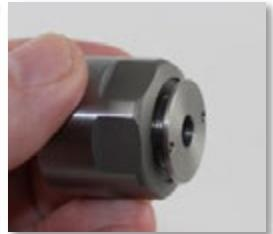
Insert cutting tool with the seal engaged on the round part of the shank, tighten cap.
